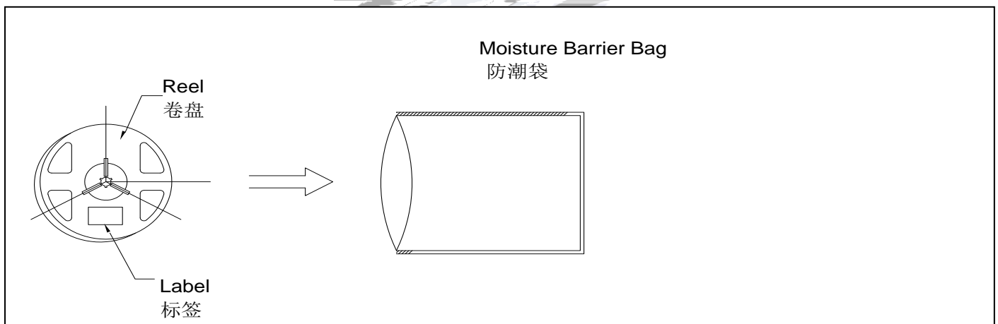
Fig.2-4 Moisture Resistant Packing 防潮包装
